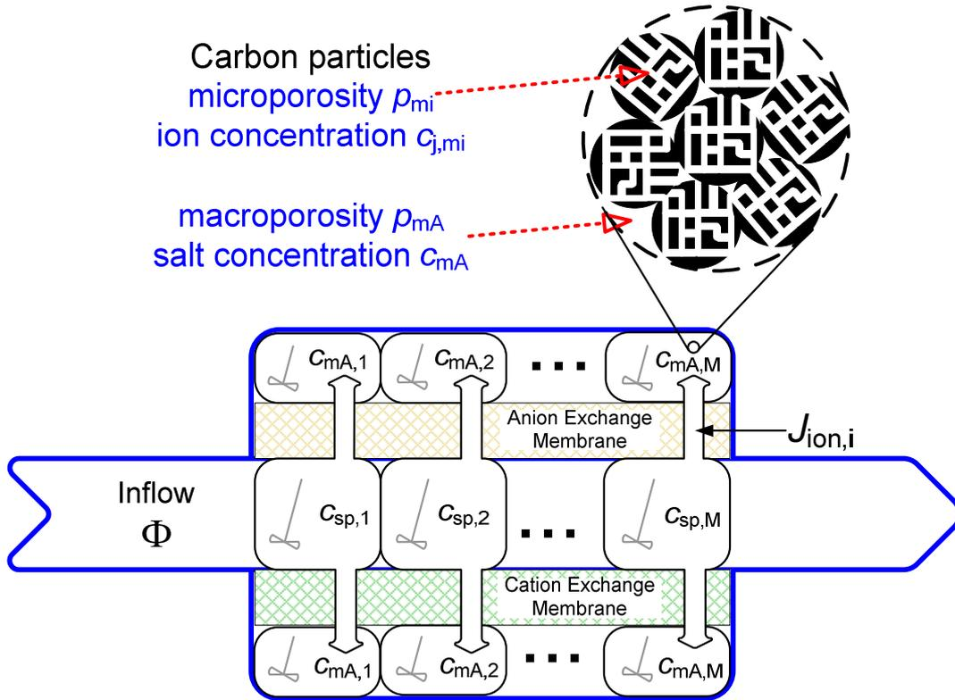
Fig. 2. Schematic view of MCDI model for ion transport and storage. Here,  $J_{ion,i}$  is the ion flux from the spacer channel into the electrode in each of the  $i=1..M$  sequential sub-cells. The electrode contains both macropores and micropores. In the macropores cat- and anions have the same concentration  $c_{mA}$ , while in the micropores the difference between cation and anion number is compensated by electronic charge present in the carbon matrix.
