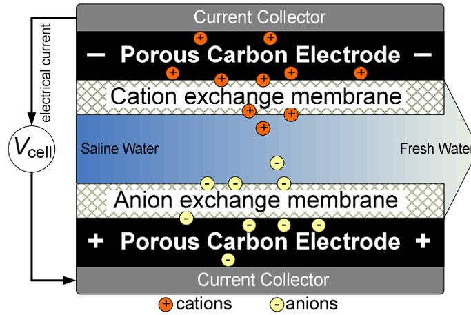
Fig. 1. Schematic view of a Membrane Capacitive Deionization-cell. By applying an electrical field, cations in the water flowing through the spacer channel migrate through the cation exchange membrane and are stored inside the adjacent porous carbon electrode (cathode) while anions are stored in the opposite electrode (anode). As a consequence, the water flowing through the cell is desalinated.
